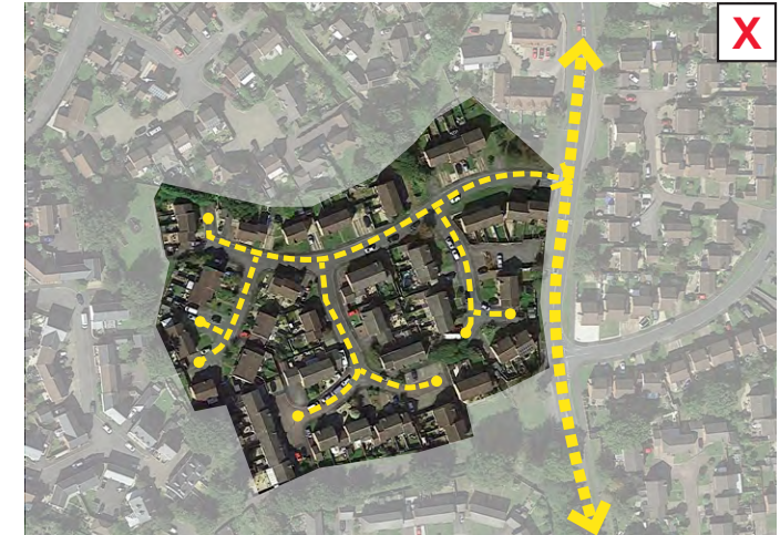
Figure 95: A layout dominated by cul-de-sacs encourages reliance on the car for local journeys. Where cul-de-sacs are used, Police guidance is that they are not connected by narrow pedestrian footpaths.
