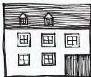
Loft conversion incorporating gabled dormers.
