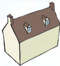
Loft conversion incorporating gabled dormers.
